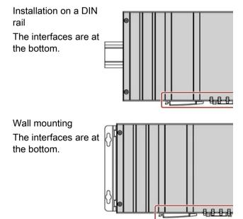
The device can be mounted vertically on DIN rails or on the wall. The figure shows the interfaces on the front.
