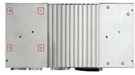
4. Insert the cover into the enclosure. Turn in the marked screws.
