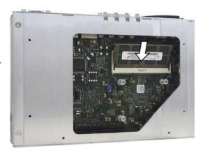
The new memory configuration is detected automatically. System RAM, extended RAM and buffer memory cache are displayed during device startup.
