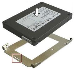
2. Insert the new HDD/SSD into the enclosure.
