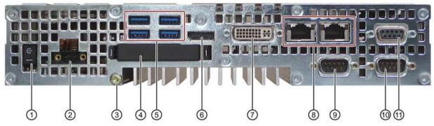
① On/off switch The on/off switch does not isolate the device from the power supply. Position "ON", when the "\_" symbol is pressed. Position "OFF" is the delivery state.
