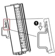
Push down the device. Once the rail clip slides over the bottom edge of the DIN rail, push the device onto the rail until it engages with an audible click.
