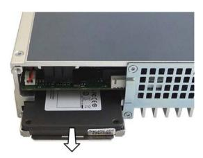
4. Loosen the HDD/SSD on the side from the base plate as shown.
