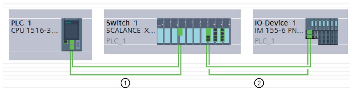
Figure 5-40 Example configuration with two rings ① and ②
