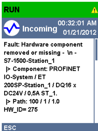
Figure 4-8 Display of alarm message
