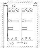
\*When units are closely mounted together, the thermal characteristics may change because of temperature increases due to the operating conditions (high ambient temperature or maximum set continuous carry current).
