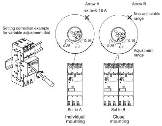
In addition, when selecting a setting near the border of the rated operating current setting range, you are recommended to select a main unit with a minimum setting that provides an adjustment margin for unnecessary operation.
