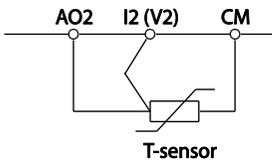
To receive PTC signal at I2 input terminal, set PRT-35 (Thermal InSrc) to '1 (V2)' and set SW 4 (Analog2 input selection switch) to V2. The sensor does not operate if SW4 is set to 'I2'.When the inverter detects a motor overheat, motor overheat trip occurs with internal delay time. The trip delay time is not reset instantly when the trip condition is released, but it only decreases as time passes.
