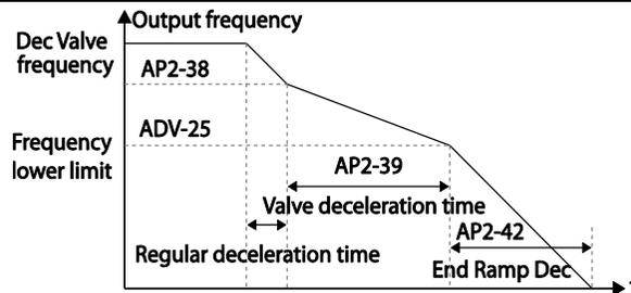
The time set at AP2-39 refers to the absolute time that it takes for the pump to decelerate from the frequency set at AP2-38 to the frequency limit set at ADV-25.
