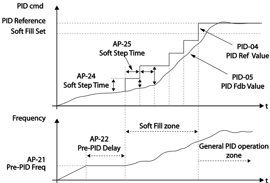
When a PID process is performed after the soft fill PID operation, the PID Reference value becomes the PID-11 PID Ref1 Set value.
