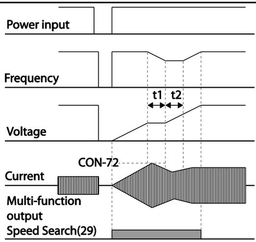
**Starting with power-on:** Set bit 4 to '1' and ADV-10 (Power-on Run) to '1 (Yes)'. If inverter input power is supplied while the inverter operation command is on, the speed search operation will accelerate the motor up to the frequency reference.
