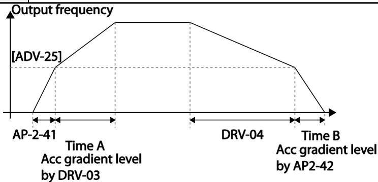
In the figure above, AP2-41 defines the acceleration time to the minimum operation frequency ADV-25 (Freq Limit Lo). AP2-42 defines the deceleration time from the minimum operation frequency to a stopped state. Time A (normal acceleration time set at DRV-03) and Time B (normal deceleration time set at DRV-04) in the figure will change according to the Acc/Dec gradients defined by AP2-41 and AP2-42.
