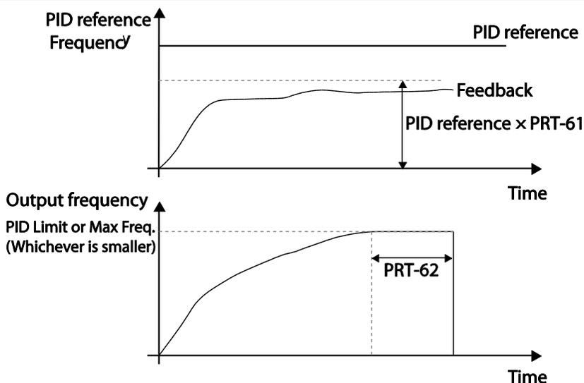
In the graph above, Pipe Break occurs if the feedback is smaller than the value calculated by multiplying the two values set at PID-04 and PRT-61(PID-04 x PRT-61) at the inverter's maximum output (when PID output is the maximum set value, or the inverter is running at the frequency set at DRV-20).
