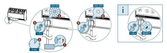
A very long push of the "programming" button of more than 20 seconds resets the device to its factory settings.
