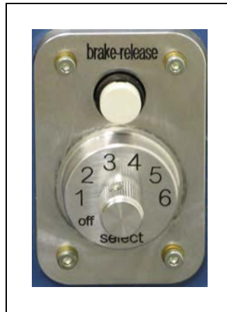
Figure 6-2. Brake Release Switch on UL Robots
