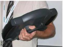
You can rest the device on your forearm, for example, to undertake movements while servicing the monitored system. The free hand can be used to operate the operator controls of the device.
