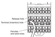
If a wire is difficult to connect because it is too thin, use a flat-blade screwdriver in the same way as when connecting stranded wire.
