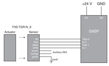
Series connection Application, up to 6 Sensors with G9SP (up to Safety PLd acc. EN ISO 13849-1)
